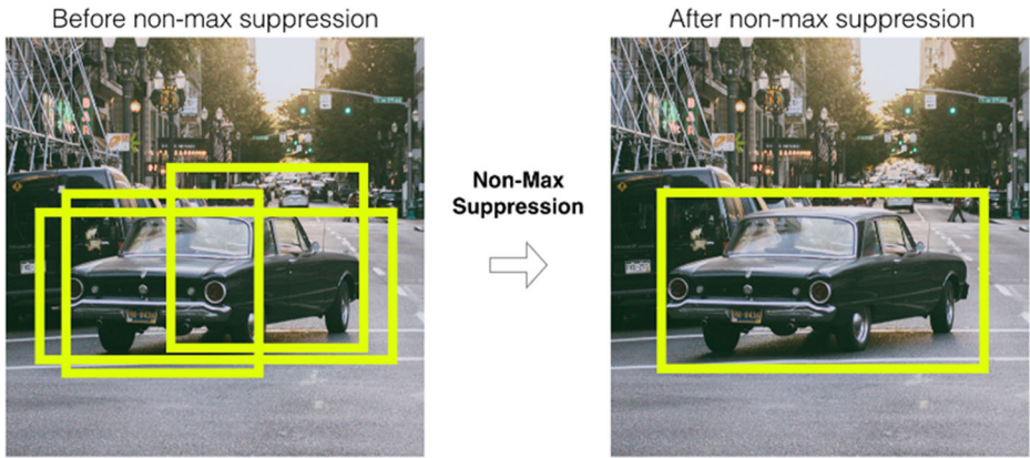
Fig. 16 The effect of Non-Max Suppression in Object detection using YOLO
