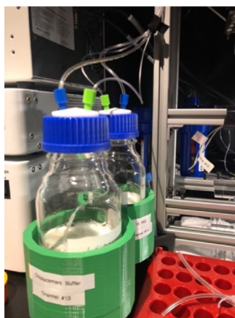
Fig. 23. Large reservoir for PBS and displacement buffer.
