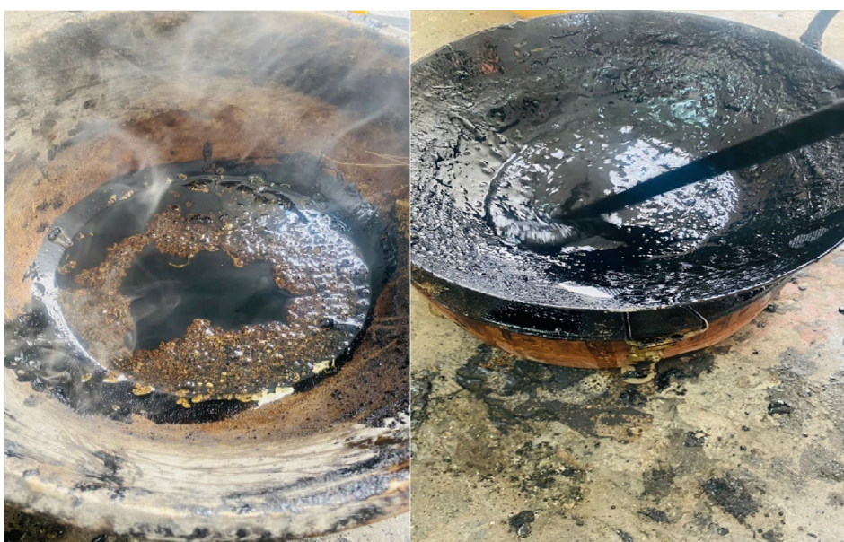
Fig. 2. (a) Thin layer of plastic in Bitumen; (b) Homogenously mixed into the Bitumen.
