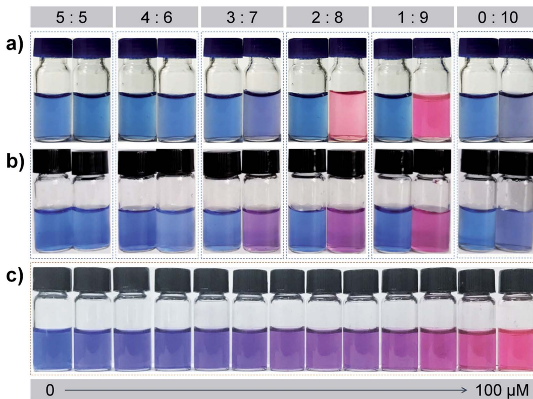
Fig. 2 Color changes of PDA liposomes prepared from (a) PCDA-EDEA-TAA and PCDA, (b) PCDA-EDEA-OA and PCDA in different mole ratios (5 : 5, 4 : 6, 3 : 7, 2 : 8, 1 : 9, 0 : 10) before and after the addition of 100 \mu\text{M} \text{Pb}^{2+} . (c) Color changes of PDA liposomes prepared from PCDA-EDEA-TAA and PCDA (1 : 9) in the presence of different concentrations of \text{Pb}^{2+} (0, 5, 10, 15, 20, 25, 30, 40, 50, 60, 70, 80, 100 \mu\text{M} ).
