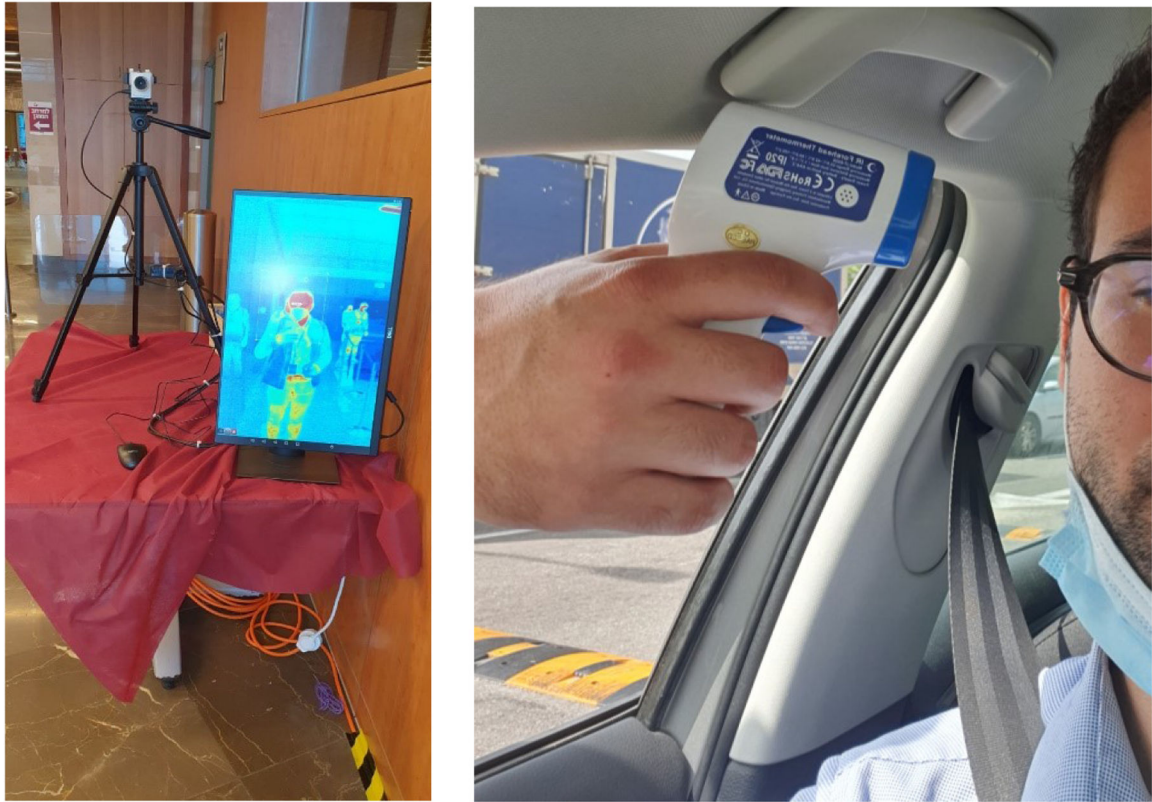
Figure 2: Point-of-contact temperature screening at the entrance of (left) a company in Israel and (right) at the entrance of the Technion Israel Institute of Technology in Haifa. Temperature may be checked using thermal imaging or non-contact infrared thermometers.
