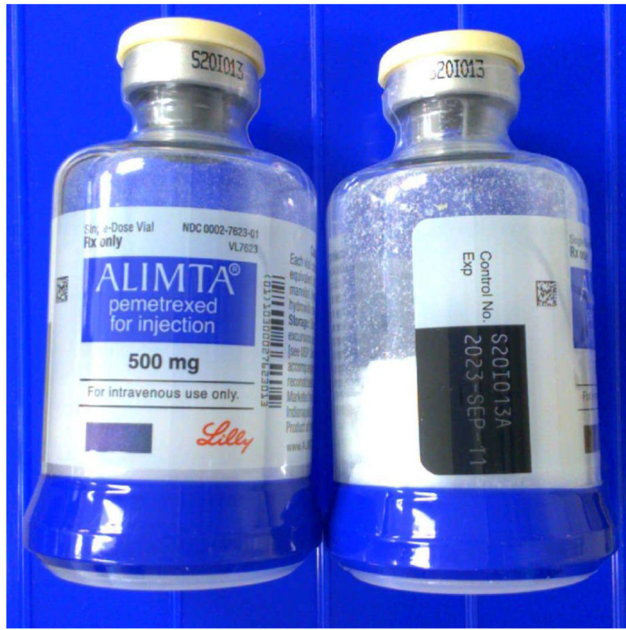
Figure 1. Vials of pemetrexed for injection. The drug appears as a white freeze-dried powder in the vial on the right. The vials were scanned in the near-infrared spectral region through the bottom of the vials.
