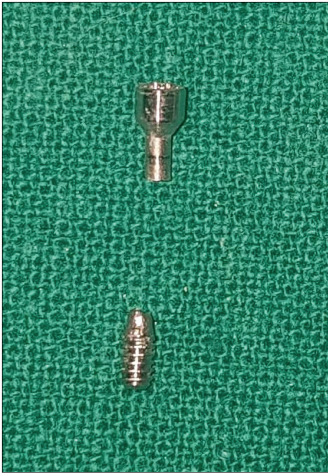
Figure 6: Retrieved fractured abutment screw fragments
