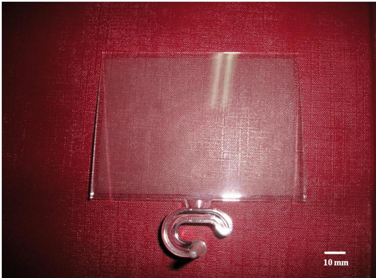
**Figure 9.** The molded light guiding plate.
