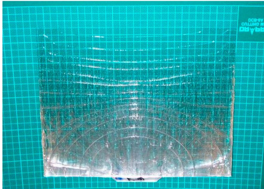
**Figure 4.** The bad flow situation of light guiding plate on micro-injection molding.
