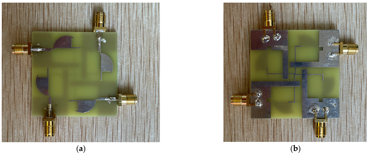
Figure 7. Photograph of the fabricated antenna: (a) top; (b) bottom.
