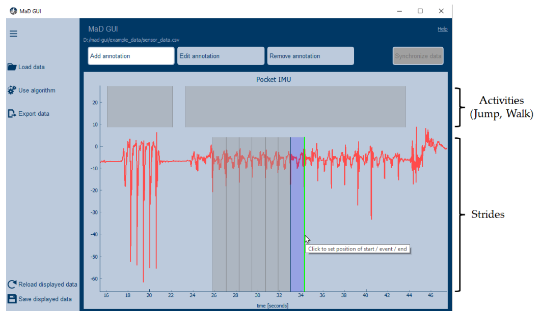
Figure 1. Main window of MaD GUI. The side-bar (left) gives access to plugins, which can be injected into the GUI. The buttons on the top change the GUI's mode, and the Add annotation mode is selected. In the upper part of the plot (first level), activities were annotated. The second level was used to annotate strides.
