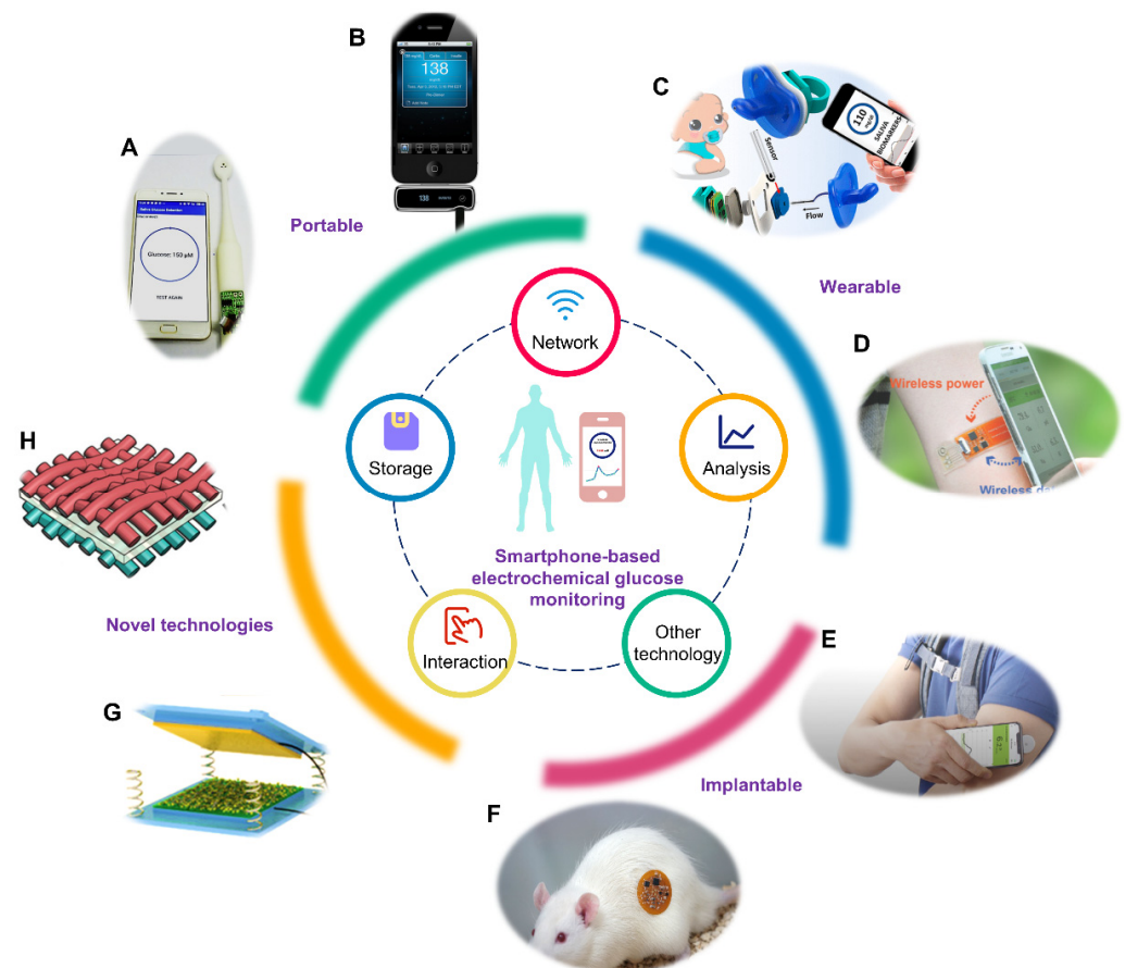
Figure 1. Smartphone-based electrochemical glucose monitoring system. The inner circle represents the technologies integrated in the smartphone. The outer circle represents the realization formats of smartphone-based electrochemical glucose monitoring and novel technologies utilized in this field. (A) Portable smart toothbrush for glucose detection in saliva. Reprinted with permission from Ref. [38] Copyright (2019) Elsevier. (B) Portable blood glucose device named iBGStar. Adapted from Ref. [39] Copyright. Medgadget, Inc. (C) Wearable saliva glucose monitoring with smartphone-based electrochemical system. Reprinted with permission from Ref. [40]. Copyright (2019) American Chemical Society. (D) Wearable sweat glucose analysis with battery-free, wireless and flexible electrochemical platform. Reprinted with permission from Ref. [20]. Copyright (2019) Wiley. (E) Implantable Free Style Libre Flash Glucose Monitoring System based on interstitial fluid produced by Abbott. Adapted from Ref. [41] Copyright Abbott Laboratories. (F) Implantable microelectrode for peritoneal glucose monitoring. Reprinted with permission from Ref. [42] Copyright (2021) Elsevier. (G) Structure of a triboelectric nanogenerator. Reprinted with permission from Ref. [43] Copyright (2019) Wiley. (H) Schematic diagram of a flexible asymmetric supercapacitor. Reprinted with permission from Ref. [44] Copyright (2020) American Chemical Society.
