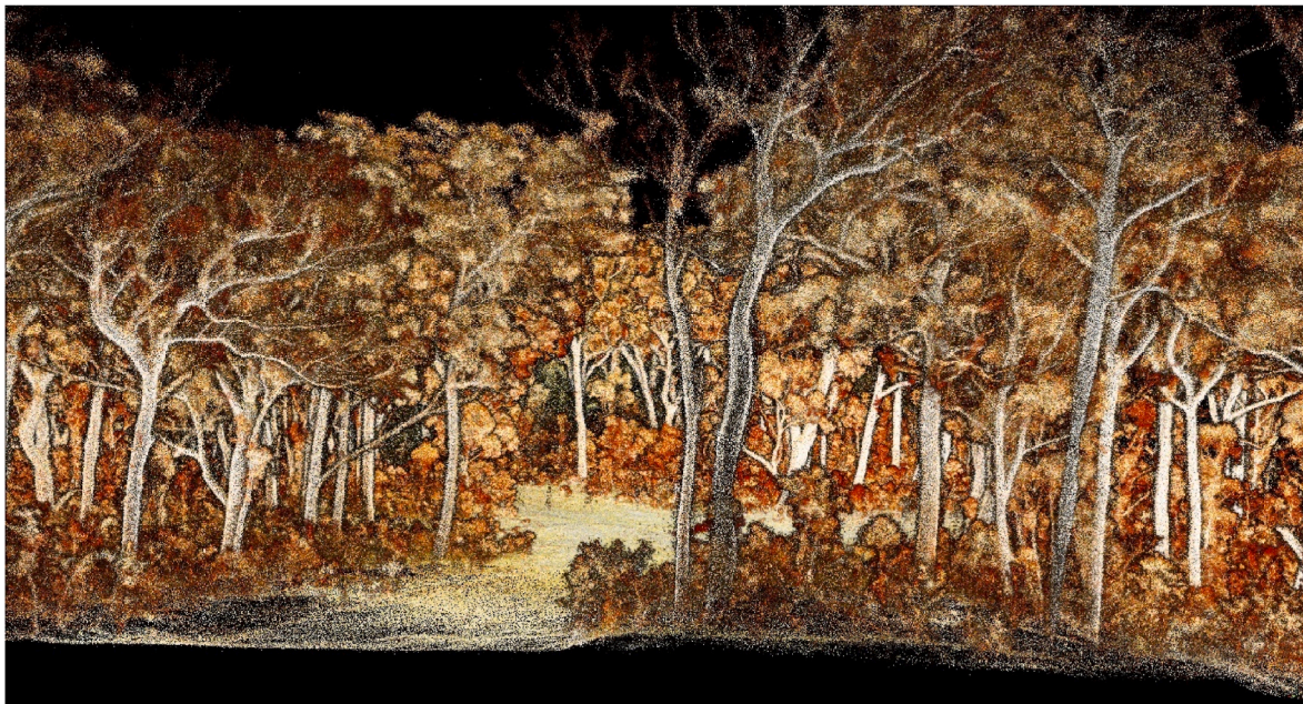
Fig. 3. – Terrestrial LiDAR capture through large, forested search areas. 3D model, captured with terrestrial LiDAR (attached to backpack), of the Belanglo State Forest in New South Wales, Australia. With similar benefits to drone-based LiDAR, this method allows for a detailed view through dense forested areas, including the potential to see mounds or depressions in the soil that could be possible clandestine graves [15]. This figure was captured using Emesent Hovermap [91] and visualized in CloudCompare [104].
