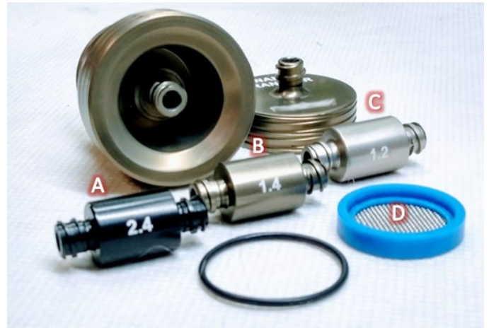
Figure 2. Adipose tissue filters A) 1.2 millimeter transfer; B) 1.4 millimeter transfer; C) 2.4 millimeter transfer; D) Mesh screen chamber (600 microns/400 microns)
