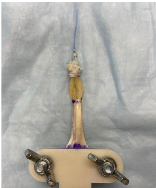
Figure 5. Decrease in tendon length at suture-tendon interface (shortening) because of the purse-string effect in a multiplanar, perpendicular looped whipstitch trial.
