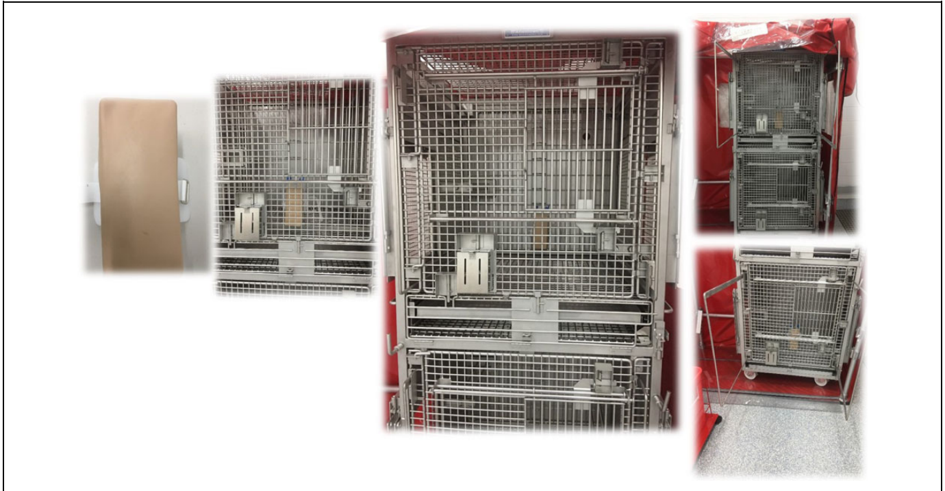
Figure 7. Mock trial setup consisting of the intramuscular (IM) simulated model and a nonhuman primate squeeze cage. The IM simulated model was strapped to the cage and squeezed to the front of the bottom and top units of the cage.
