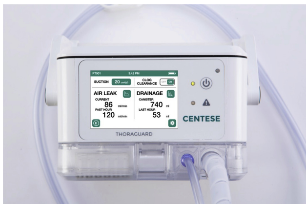
FIGURE 4. Thoraguard Control Module. An electronic monitor that provides the core functionality of the Thoraguard System. It incorporates an integrated pump, battery-power, sensors for suction regulation, and digital measurements of fluid output and air leak rate.
