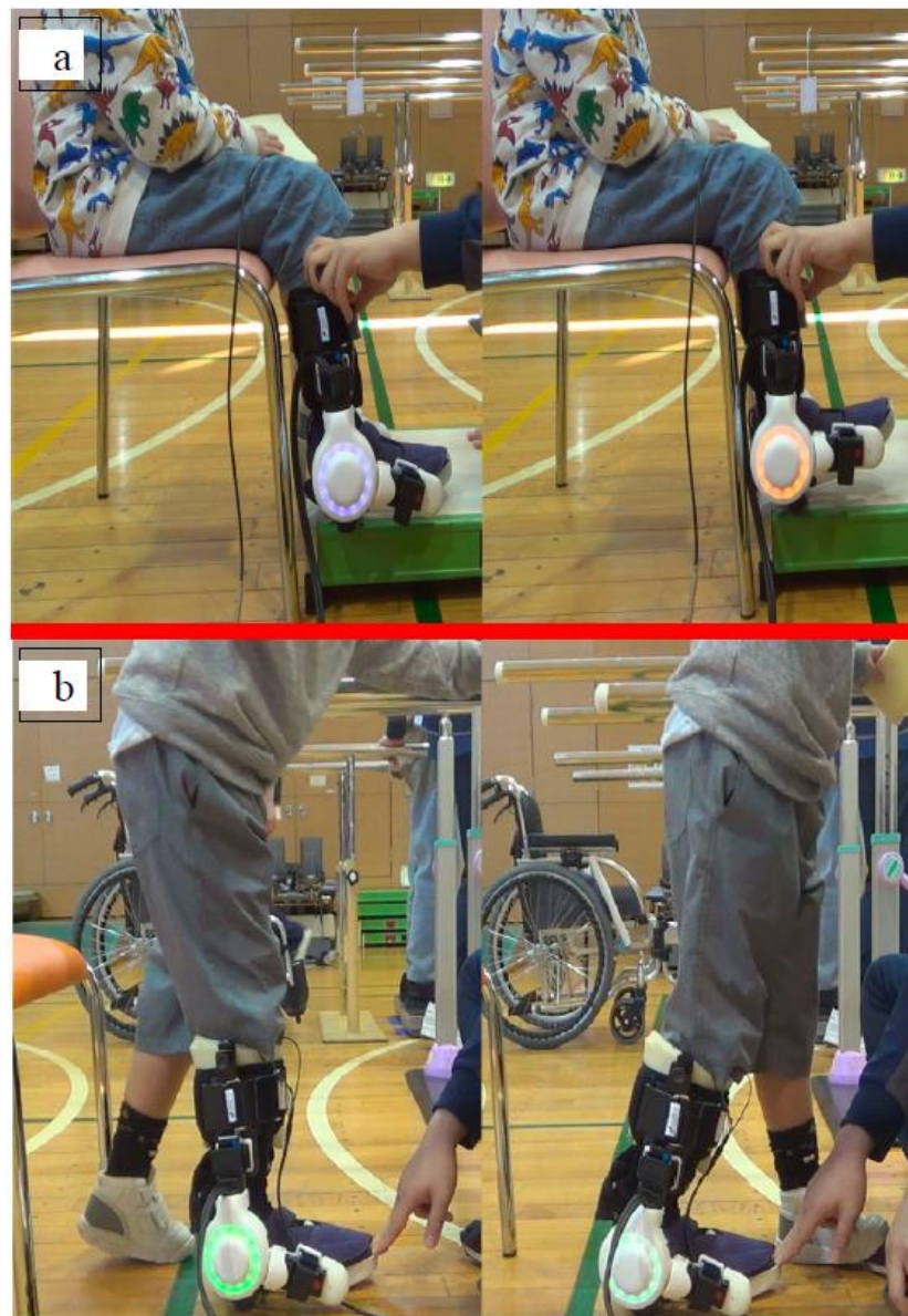
Figure 5. Single-joint Hybrid Assistive Limb (HAL-SJ) training: (a) dorsiflexion exercise and (b) stepping exercise.
