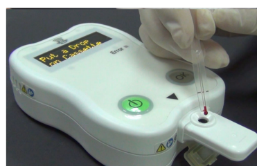
Figure 2. Physical photograph of the iProtein immunoassay and SH-SAW sensor chip coated with SARS-CoV-2 S protein.
