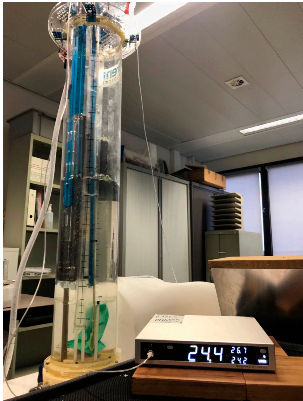
Figure 4. The Spiegelberg measurement device (Spiegelberg GmbH, Hamburg, Germany) showing the mean, maximal, and minimal IAP values (in mmHg).
