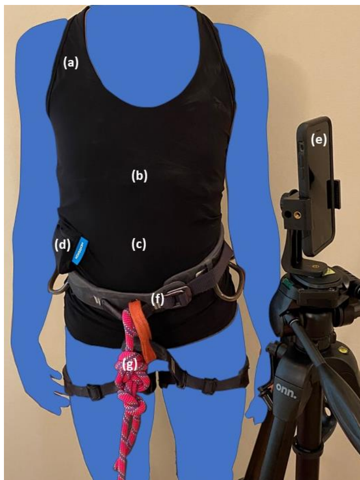
Figure 1. Setup for collecting biometrics and video of a lead climb, which includes: (a) biometric compression shirt; (b,c) thoracic and abdominal bands with respiratory and cardiac sensors; (d) compression shirt pouch with data logger and accelerometer; (e) smartphone for climbing video; (f) climbing harness; and (g) climbing rope.
