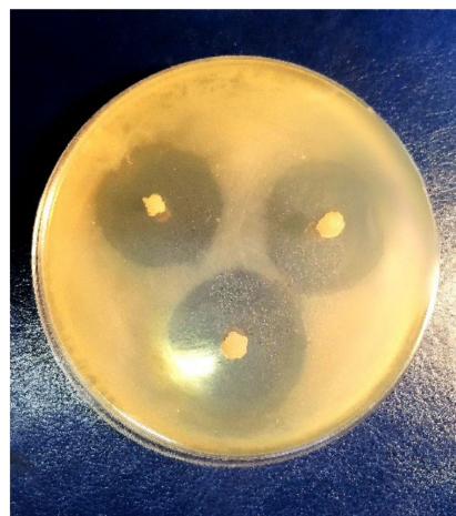
Figure 12. Growth-inhibition zones for the E. coli cells around the DON loaded Ca(ALG/CNS) sponge carrier (2 in Table 1) after 24 h of incubation.
