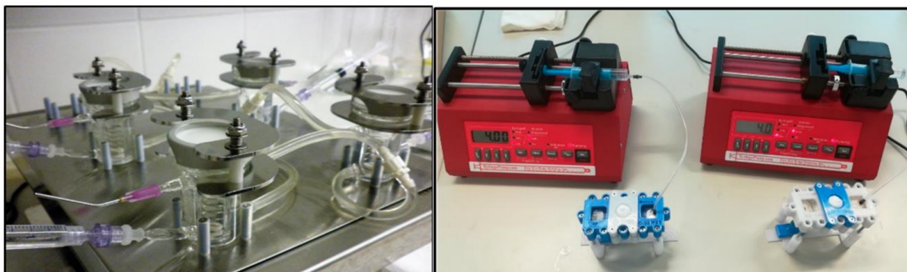
Figure 3. The static Franz diffusion cells ( left ) and the dynamic skin-on-a-chips ( right ). Both in the Franz cell and the skin-on-a-chip, the direction of the diffusion is vertical, but while in the Franz cell there is continuous stirring with a helical stirrer, in the chip, there is a continuous flow of the perfusion fluid below the skin sample.
