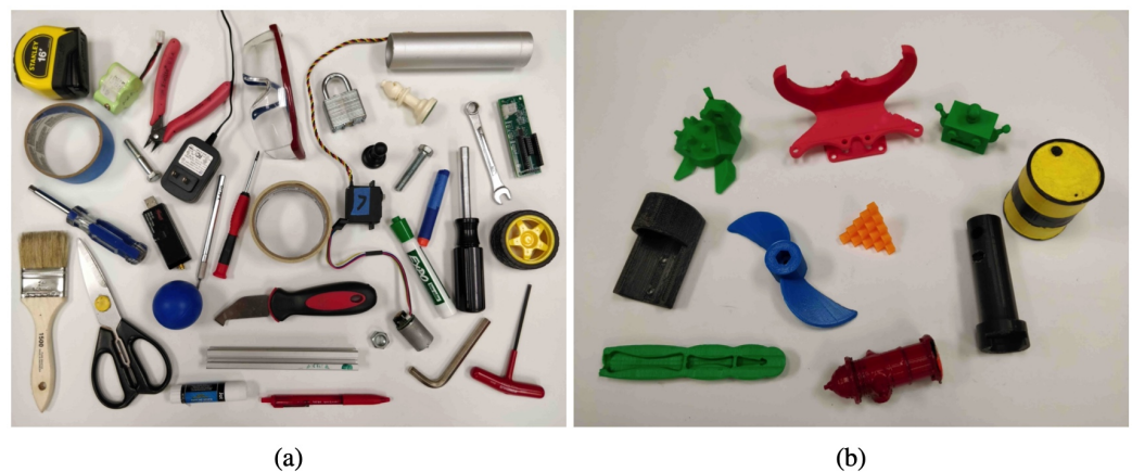
Figure 13. Objects used for robotic grasping experiments. (a) Household test objects. (b) Adversarial test objects.
