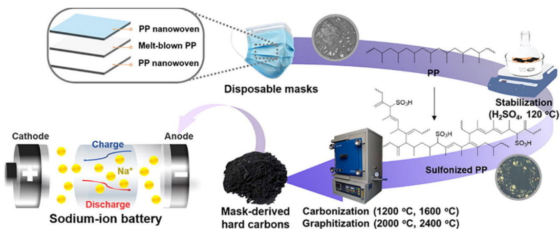
Fig. 8. Schematic representation of HC synthesis from FMWs for anodes in Na-ion batteries. Reprinted with permission from Ref. Lee et al. (2022). (Copyright 2021, Elsevier).
