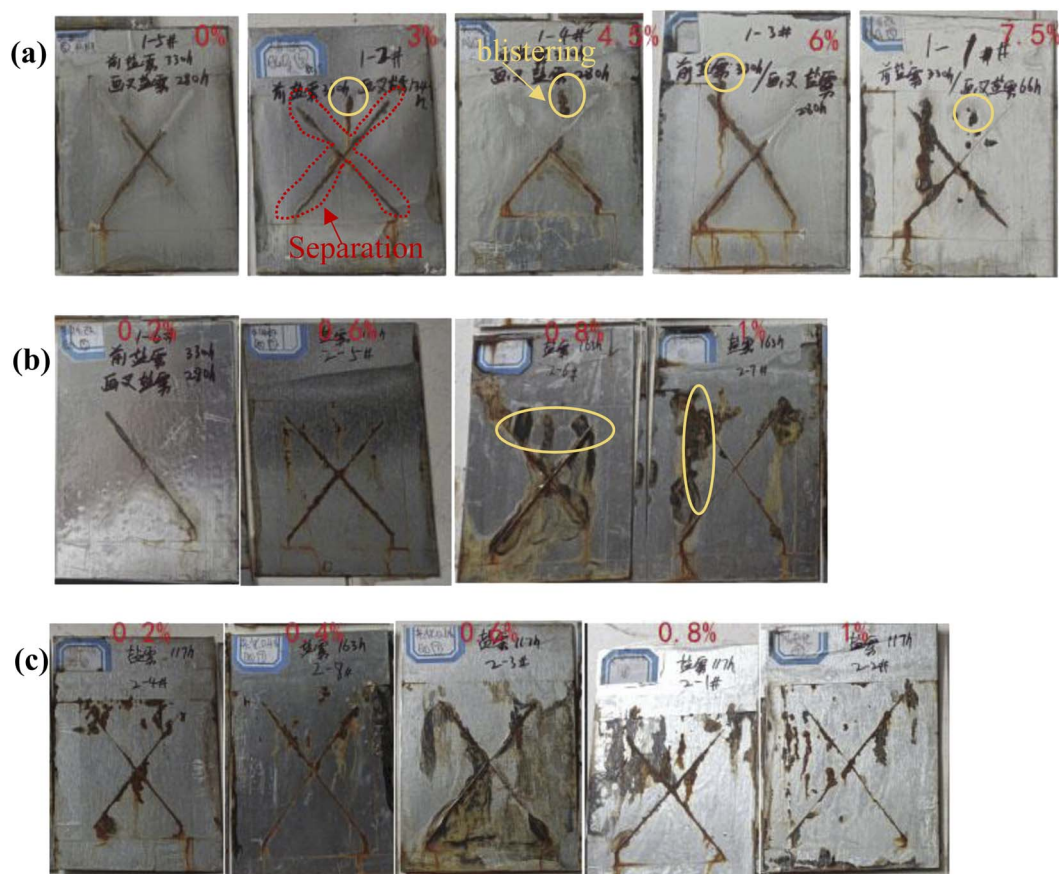
Fig. 12 Digital images of the composite coatings containing (a) m\text{-Al}_2\text{O}_3 , (b) mGO and (c) m\text{-Al}_2\text{O}_3\text{@GO} hybrids after exposure to salt spray test.
