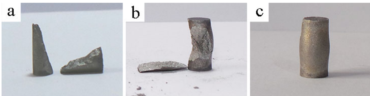
Figure 3. Low-magnification images of the specimens after compression at (a) up to 150 °C, (b) 250 °C, and (c) 350 °C.
