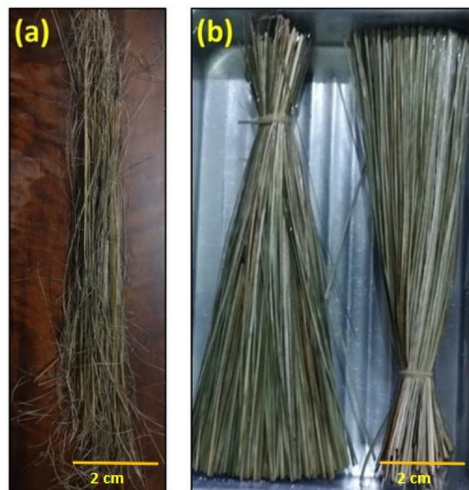
Figure 1. (a) Sedge fibers as received; (b) sedge fibers immersed in water for 24 h.
