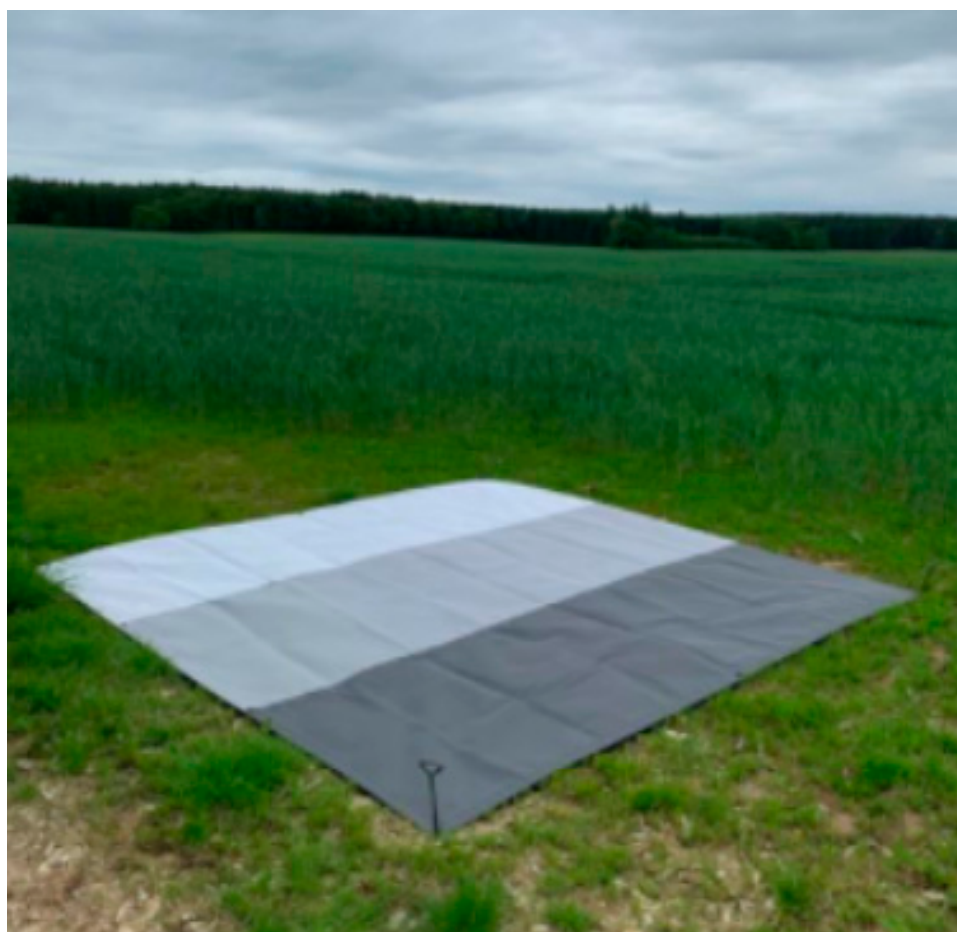
Figure 8. Tarp with the three gray reflection levels deployed at the interest area, used for radiometric calibration.
