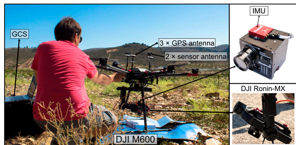
Figure 3. Setup of the DJI Matrice 600 UAV system and Nano-Hyperspectral sensor. The computer on the figure's left side is used as ground control station (GCS), allowing to control all mission's operations.
