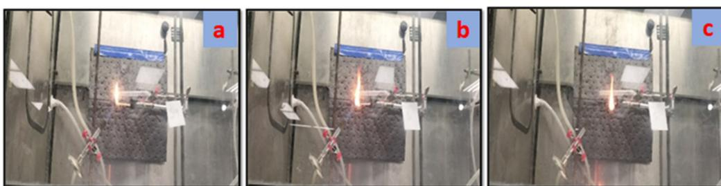
**Figure 9.** (a) Lighting of composite sample, (b) Distance of 25 mm traveled by the flame in T1, (c) Distance of 60 mm traveled by the flame in T2.
