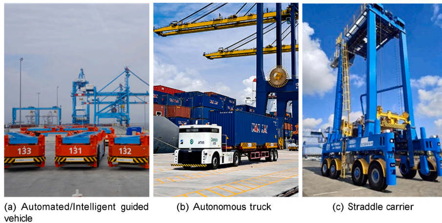
Fig. 4. Illustration of terminal transport vehicles. (a) Automated/Intelligent guided vehicle, (b) Autonomous truck, (c) Straddle carrier.
