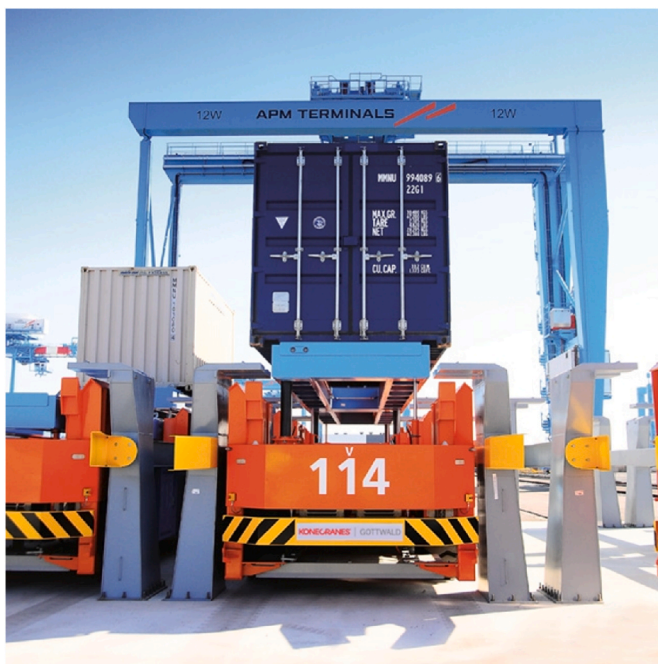
Fig. 5. Illustration of lifting AGV by Konecranes.
