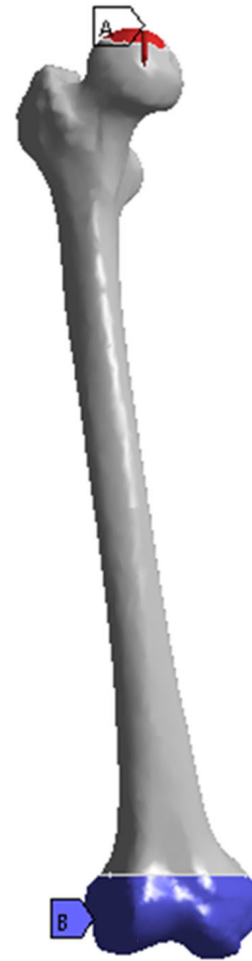
FIGURE 5 Set the 30 mm diameter range above the femoral head as the loading surface, and set the femoral condyle as the restraining surface
