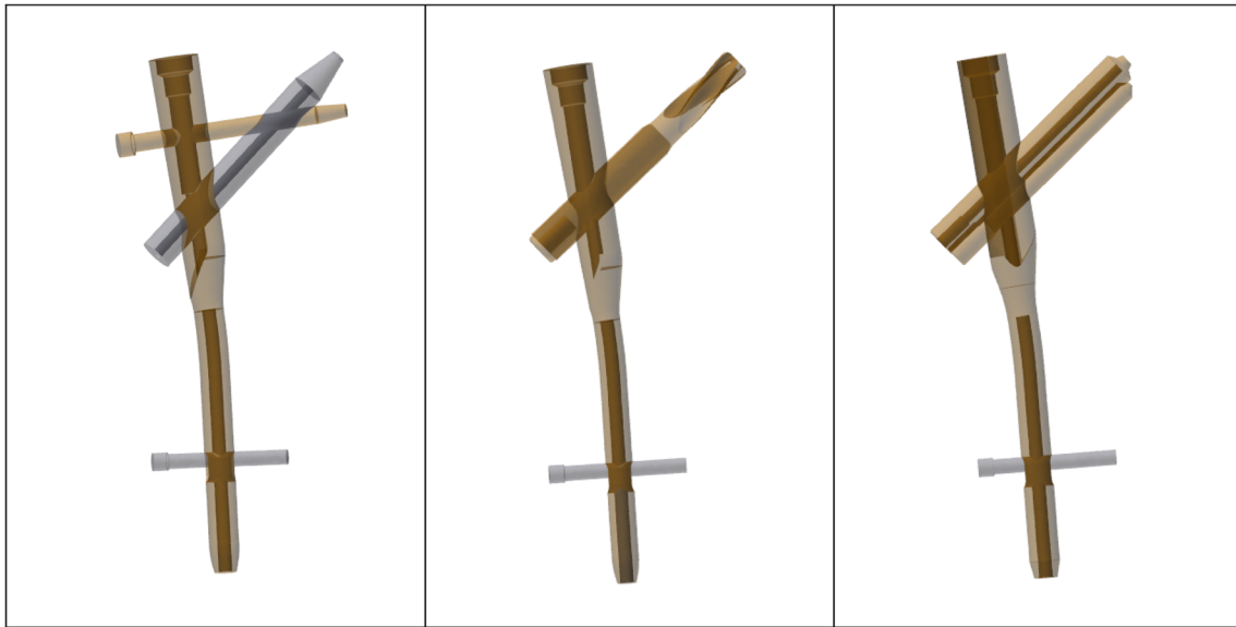
FIGURE 2 The three-dimensional geometric model of proximal femur bionic nail (PFBN), proximal femoral nail antirotation (PFNA) and InterTan
