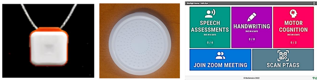
Figure 1. IADLSys: a pendant sensor (PAMSys+, left); wireless tag (pTAG, middle); and interaction-tablet PC (right).
