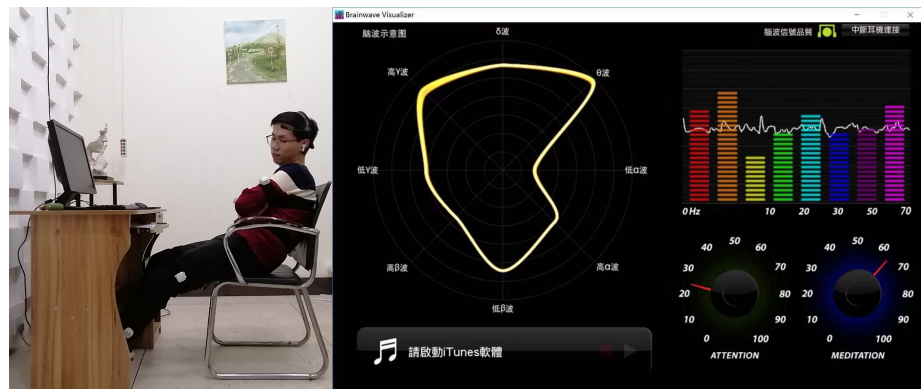
Figure 18. Brainwave Visualizer. The EEG signals, “Attention”, and “Meditation” of listening to music at 3000 k–300 lx.
