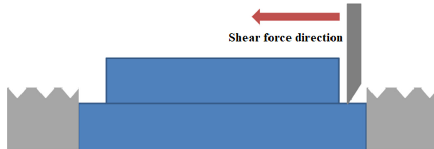
Figure 8. Schematic diagram of shear force test.
