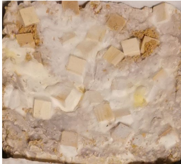
Figure 3. Sample based on hemp mix with wood cubes. Surface: smooth with inclusions; color: off-white, wood inclusions (photo A. Bonenberg).
