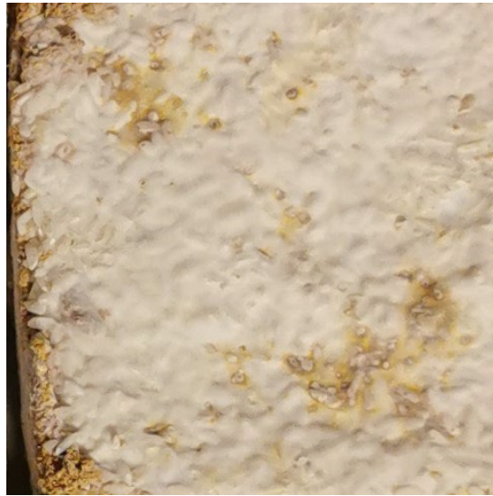
Figure 1. Sample based on hemp mix with rice. Surface: smooth, with grains of rice and substrate fibers; color: off-white, with irregularities (photo A. Bonenberg).
