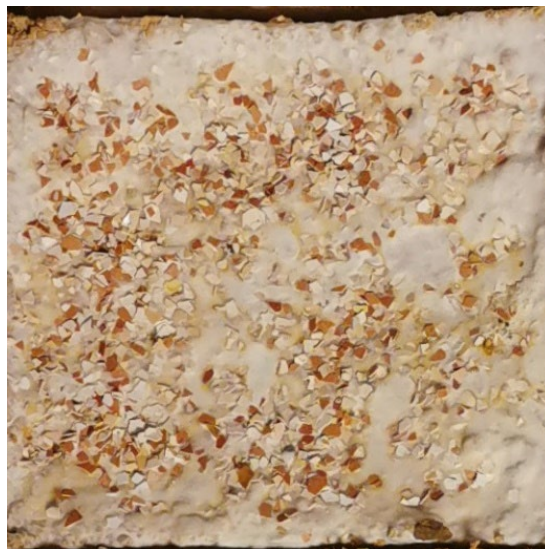
Figure 4. Sample based on hemp mix with eggshell. Surface: smooth with eggshell. Color: off-white mycelium, gray, eggshells (photo A. Bonenberg).
