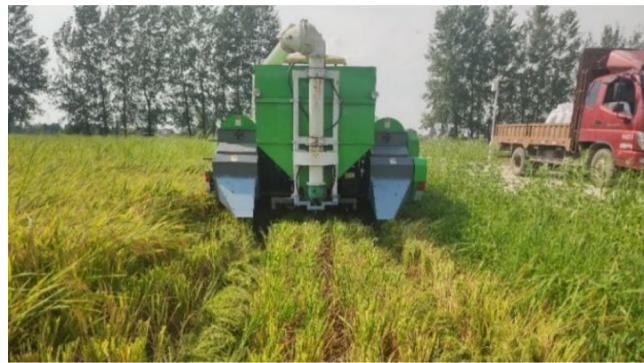
Figure 8. Field test of smashing and scattering device.
