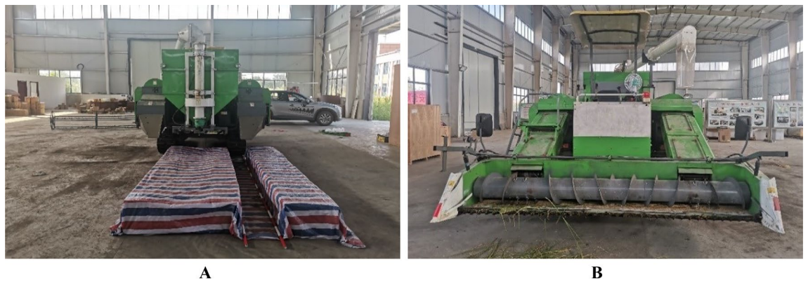
Figure 7. Bench test of smashed straw scattering. (A) simulation of rolling and stubble area, (B) feeding inlet.
