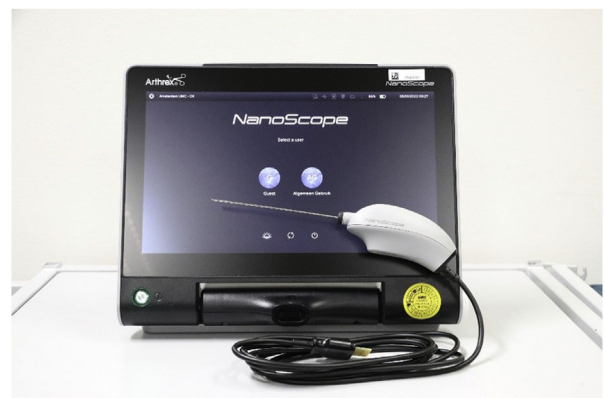
Fig 2. The needle arthroscopic set consists of the portable video console and the handpiece set.
