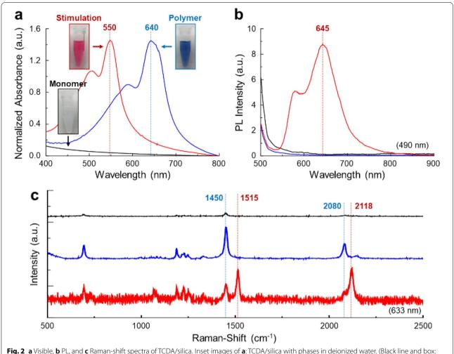
Fig. 2 a Visible, b PL, and c Raman-shift spectra of TCDA/silica. Inset images of a: TCDA/silica with phases in deionized water. (Black line and box: monomeric phase, blue line and box: polymeric phase, and red line and box: thermal stimulated phase (~110 °C))
