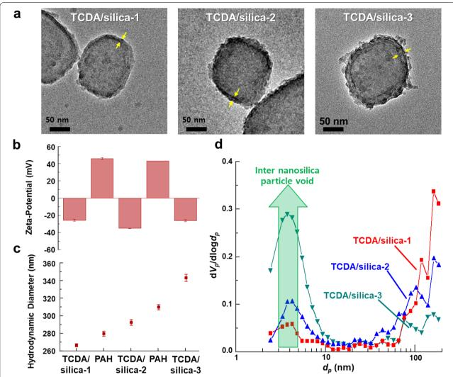
Fig. 5 a TEM images, **b** Surface charge and **c** HDD of monomeric TCDA vesicles with repeated silica armor membranes. **d** Brunauer–Emmett–Teller (BET) analysis results of the silica armor membranes on monomeric TCDA vesicles. The n value of PCDA/silica-n indicates the number of silica armor membranes
