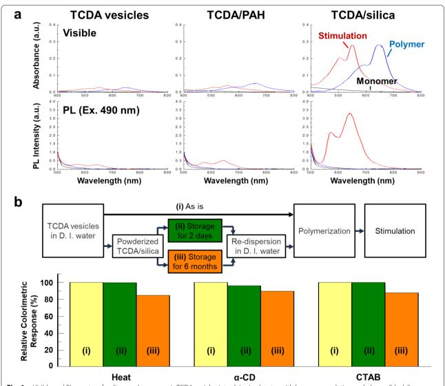
**Fig. 4** a Visible and PL spectra of redispersed monomeric TCDA vesicles into deionized water with layer encapsulation and phases (black line: monomeric phase, blue line: polymeric phase, and red line: thermal stimulated phase (~110 °C)), **b** Sustainable sensing response of TCDA vesicles with layer encapsulation. Relative CR values of reactivity test of (i) unstored TCDA vesicles and redispersed TCDA/silica after (ii) 2 days and (iii) 6 months
