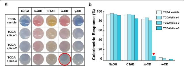
**Fig. 6** Size-selective recognition of TCDA vesicles in silica armor membranes. **a** Photo-images and **b** colorimetric response values of TCDA vesicle in silica membrane with 10 mM of chemical stimuli. The CR value of PCDA/silica-3 lowered significantly in response to α-CD (red highlight). The n value of PCDA/silica-n indicates the number of silica armor membranes
