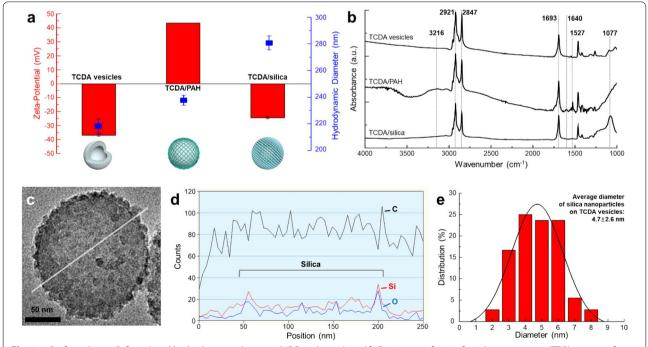
Fig. 1 a Surface charge (left axis) and hydrodynamic diameter (HDD, right axis), and **b** Fourier transform infrared spectroscopy (FTIR) spectra of 10,12-Tricosadiynoic acid (TCDA) vesicles with different surface layers. **c** Transmission electron microscopy (TEM) image of monomeric TCDA/silica and **d** Energy dispersive spectroscopy (EDS) spectra of section shown by the white line in **c**. **e** Size distribution of silica nanoparticles on the TCDA vesicles
