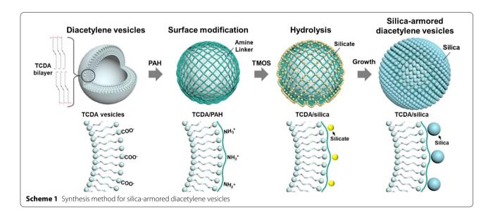
optical responses. These pores can be controlled using an electrostatic LbL approach [26, 27] and the direct hydrolysis of silica, which can form continuous dense silica nanoparticles. By repeating this process, porous membranes of varying thicknesses can be formed on vesicles. The membrane permeability depends on its thickness; and we developed a size-selective recognition function for PDA vesicles with different stimulating molecules/structures.
