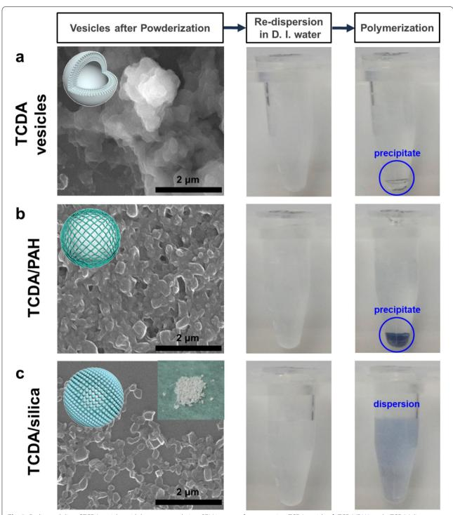
**Fig. 3** Redispersibility of TCDA vesicles with layer encapsulation. SEM images of monomeric **a** TCDA vesicles, **b** TCDA/PAH, and **c** TCDA/silica after powderization (Inset image of **c**: TCDA/silica powder), and photo images of the sonicated monomeric powders into deionized water and its polymeric phase
