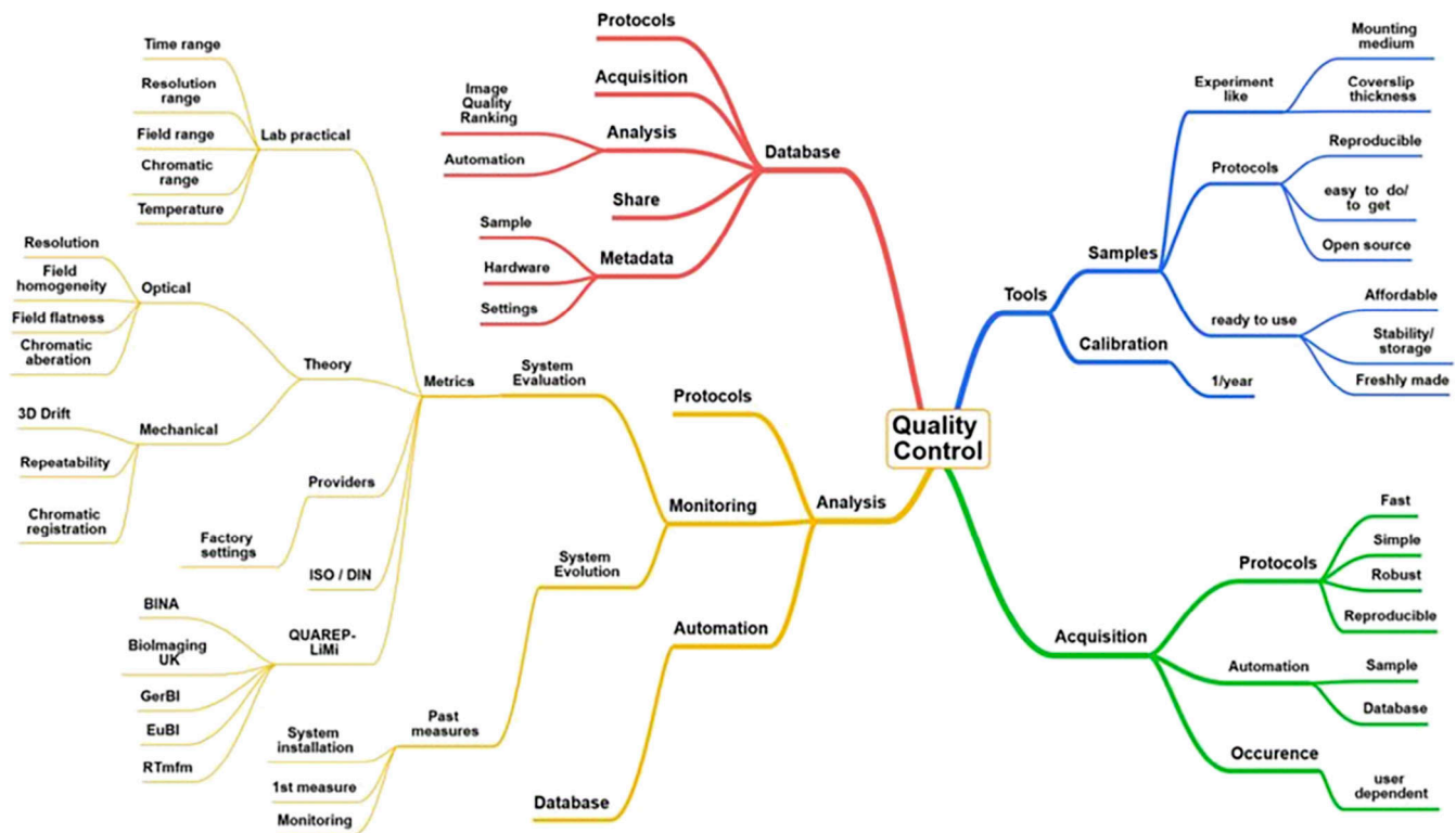
Figure 10. Heuristic map of light microscopy QC. QC needs tools (blue branch), acquisition protocols (green branch), image analysis (yellow branch), and clever data storage (red branch).
