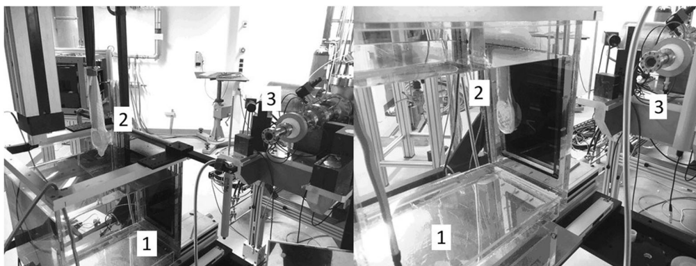
FIGURE 5 Experimental setup at PTB (Germany). Both images show the water tank (1), the UTIC (2) in a waterproof bag mounted on a xyz positioning system outside water (left) and in the water at reference depth (right) and the beam exit window of the beamline of the electron linear accelerator (3)
