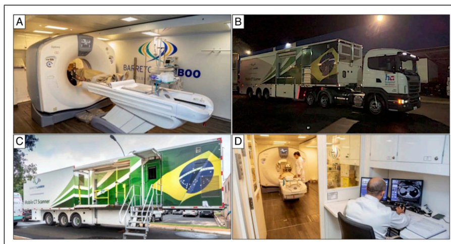
Figure 1. The Mobile CT Unit: (A) inside view of the operational CT room; (B) Mobile CT unit in displacement; (C) external lateral view, with the CT room already expanded on the back, the hydraulic elevator, and the entrance latter on its right, and (D) inside view of the CT room from the command room.
