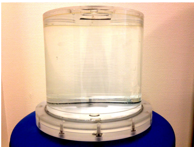
FIG. 1. Cylindrical water tank phantom. Diameter: 20 cm; length: 25 cm. [Color figure can be viewed at wileyonlinelibrary.com ]
