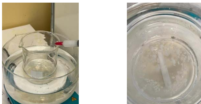
Figure 2. Performing the microencapsulation of essential oils in a sodium alginate shell.
