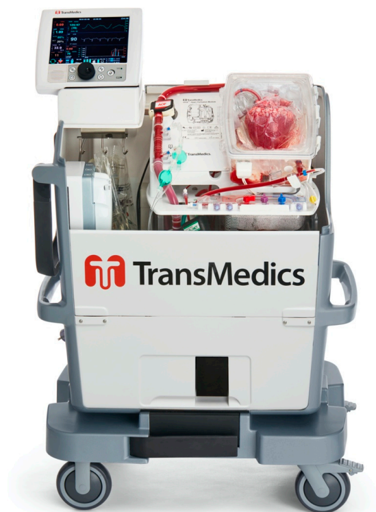
Figure 2. Transmedics Organ Care System. Normothermic, continuous perfusion is established via the aortic root. The heart is maintained in sinus rhythm during transport. Photograph used with permission from Transmedics Inc.
