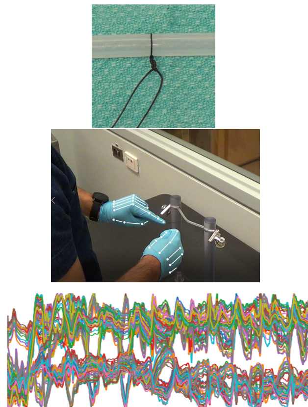
Figure 1. The trials were recorded using three modalities. The top is an image of the final product, the middle is a screen capture of the video data with a visualization of the joints tracked by the Leap sensor. The bottom is an example of the kinematic time series data, representing the temporal 3-dimensional movement of the hand joints during the knot tying task.
