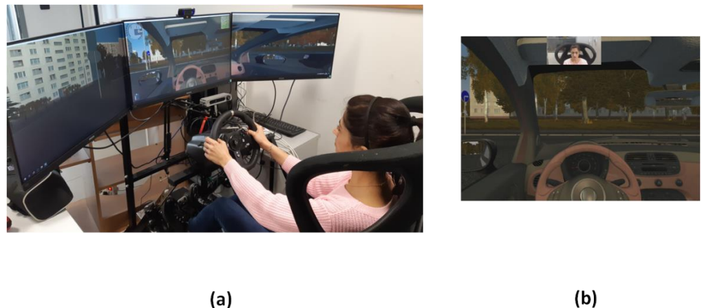
Figure 1. Experimental setting: (a) static driver simulator; (b) screenshot of the driving simulation software (i.e., City Car Driving, Home Edition software-version 1.5, Forward Development, Ltd., Verona (WI), USA [37]).
