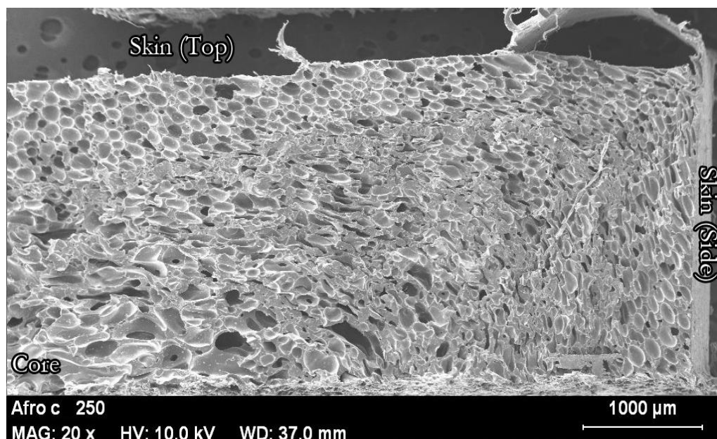
Figure 13. Sample with a relative density of 0.2 and produced with 10.5% of azodicarbonamide. Near the skin the cellular structure shows a regular structure. 500 \mu\text{m} from the skin, several cells are crushed in the direction from the core to the skin. In the core, the cells are four times larger than in the skin.
