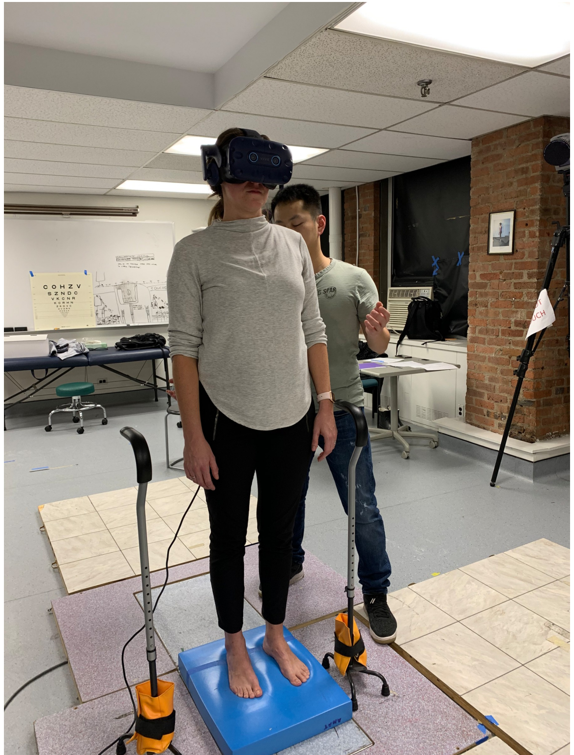
Fig 1. Experimental setup when a participant is standing on memory foam.
