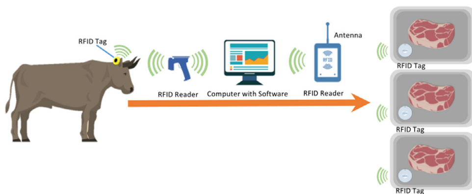
Fig. 2. (a) The monitoring system of livestock which is based on RFID. (b) RFID tags applied in the food industry.
