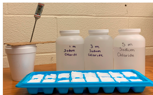
Figure 1. Photograph of thermal calorimetry apparatus used in the first experiment (part A) of this activity. The image also includes the frozen salt cubes, shown in a food-grade ice-cube tray, as well as bottles of chilled aqueous salt solutions.
